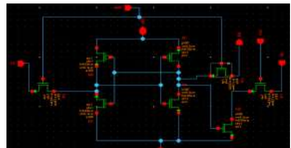
Fig.11: schematic representation of 8T SRAM
